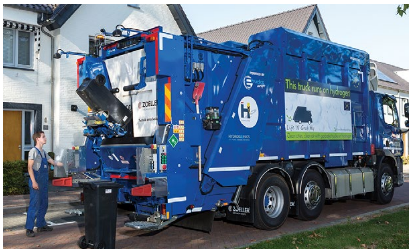
Pilot project with a waste collection vehicle running on hydrogen. © Waterstofnet
